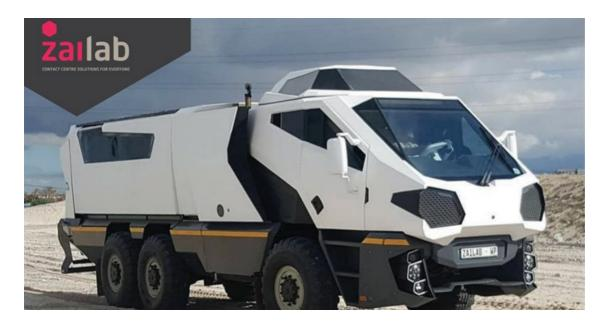
The custom-built vehicle features a repurposed military 6×6 MAN KAT chassis, while the bodywork design was inspired by futuristic vehicles from science fiction films such as *Tron, 2001: A Space Odyssey* and *Star Wars*, as well as a heavy duty V10 diesel engine. The truck can survive even the toughest terrain, which has come in handy in its great trek across the continent.
