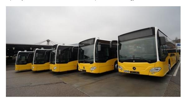
"The objective with the Citaro hybrid is to make the diesel engine even more economical while optimising the degree of electrification for maximum overall economic efficiency," says Rüdiger Kappel, sales manager Mercedes-Benz Buses Germany, explaining the concept behind the vehicles. A disc-shaped electric motor is positioned between the engine and the automatic transmission.
