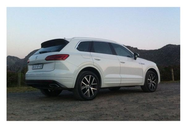
The new dimensions: 4,878 mm length (+77 mm), 1,984 mm width (+44 mm) and 1,702 mm height (-7 mm). The increase in length and width in conjunction with the slightly reduced height leads to significantly more dynamic proportions, yet still looking classy as ever.
