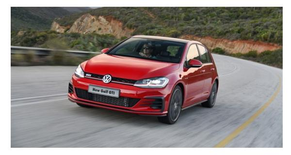
The most noticeable visual change is a narrower grille and headlights which stretch into the bumpers, a strip of small daytime LED lights up front and LED main lights on some of the more expensive models.
