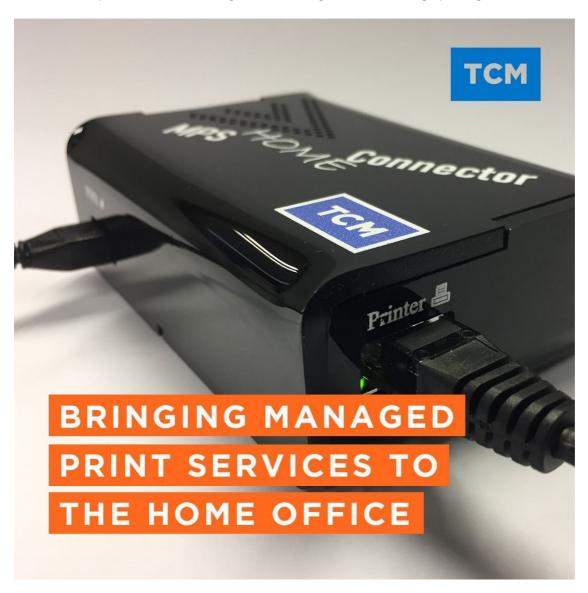
MPS Connector is a managed printing service connector device that integrates directly and securely into existing MPS management platforms to enable the full automation and reporting centralisation of a remote fleet. The technology will provide employees that are working from home the same level of print service they have become accustomed to in the corporate workplace.
