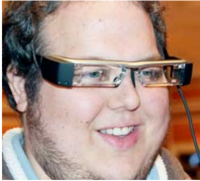
Clunky glasses known as the Moverio BT-200 and made by Seiko-Epson are aimed at real applications ranging from aircraft inspections to medical assessments. Image: GizMag
