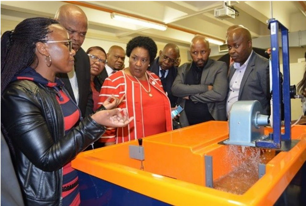
From L-R Ms Kekeletso Thejane, Assistant Lecturer and master's student at Department of Mechanical and Mechatronics Engineering demonstrating the Pelton wheel turbine machine to the FSPG delegates. The machine is driven by the jet of water which is supplied by the pump from the hydraulic bench. The water strikes the buckets to rotate and produce a torque and power to produce the electricity.
