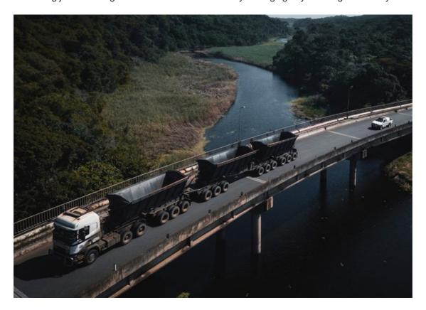
PBS vehicles bring a myriad of advantages to the mining sector. Customised designs tailored to specific operational requirements enable enhanced payload capacity, reducing the number of trips needed for transportation. This translates into cost savings and minimises the environmental footprint associated with fuel consumption and emissions. This improved efficiency in transporting bulk materials contributes to a streamlined supply chain, ensuring timely deliveries and sustained production.
