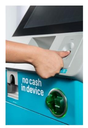
Known as TouchPoint, the device functions as a self-service kiosk from which customers can conduct transactional banking such as withdrawals, transfers and payments, view statements, purchase airtime and electricity and perform card cancellations. In addition to this, the device also allows for new account opening by reading a consumer's thumb print.
