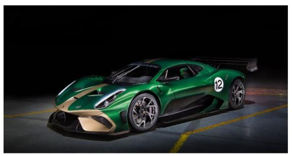
The Brabham BT62 weighs in at a mere 972 kilograms and has a huge 5.4-litre V8 that outputs 522 kW and 667Nm of torque (Oredit: Brabham)
